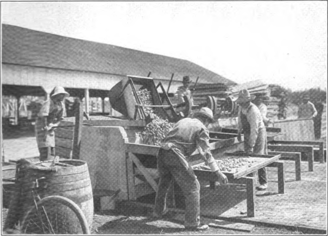
Washing and cleaning the dried Calimyrna Figs in a salt and baking soda solution.
