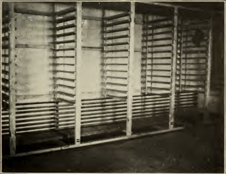
FIG. 2.—INTERIOR OF OVEN FOR DRYING TRAYS OF FIGS WHICH HAVE BEEN STERILIZED BY BOILING, USED IN A FIG "KHAN" IN SMYRNA. (ORIGINAL.)
