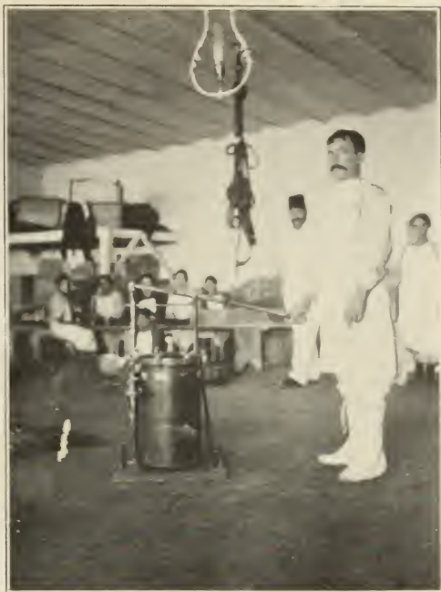
FIG. 1.—A HAND VACUUM MACHINE FOR EXTRACTING AIR FROM JARS OF FIGS, AND ITS OPERATOR.
