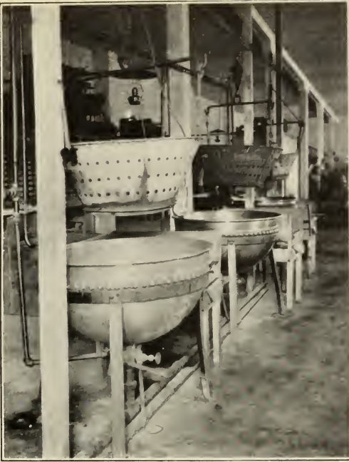
FIG. 1.—COPPER BOILERS AND GALVANIZED STRAINERS USED FOR STERILIZING FIGS IN A SMYRNA "KHAN." THE PERCENTAGE OF LIVING LARVÆ IN THE FIGS IS MUCH REDUCED BY SCALDING. (ORIGINAL.)
